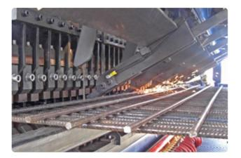
Versatility is at the heart of the AMM II, effortlessly processing cold- or hot-rolled materials ranging from 4mm to 20mm from coil. Its intelligent automation adapts to specific production requirements, including the ability to weld different line and cross-wire diameters within the same mesh. This capability allows for the creation of highly customized and diverse products.
