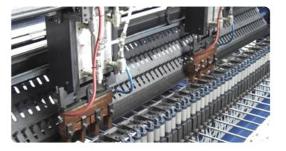
A key advantage of the AMM XY is its ability to weld different line and cross-wire diameters within the same mesh, providing unmatched customization. Programmable cross-wire placement, ensures that users can achieve multiple cross-wire spacing options within a single mesh, delivering a level of precision and versatility that sets it apart from conventional systems.
