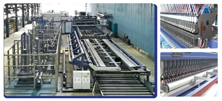
Equipped with full welding heads and twin-wire feeding for both line and cross wires, the AMM II synergizing with the Flexi-Line Twin series straightening machine, to deliver superior productivity, surpassing conventional mesh welding lines.
